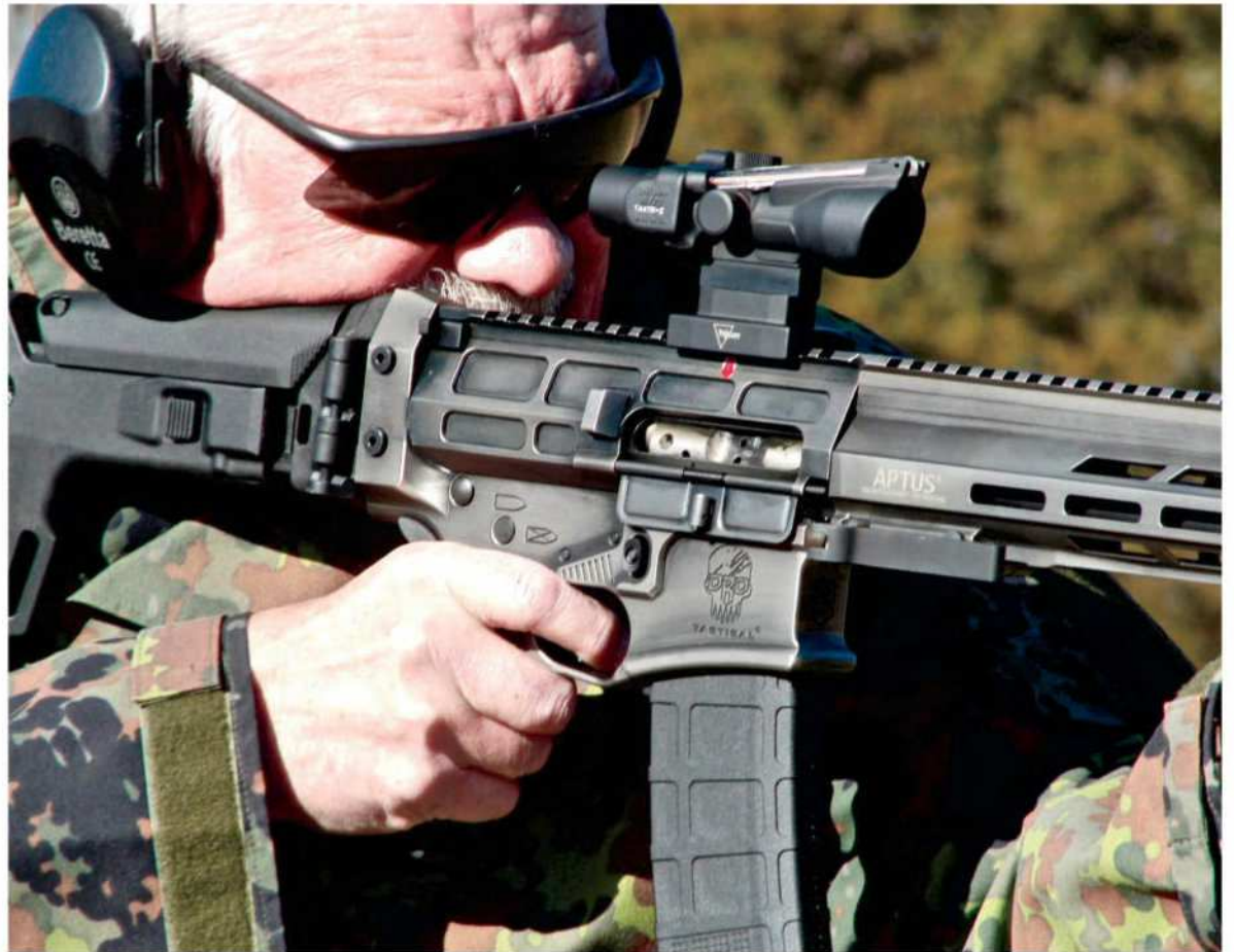
Engaging offhandedly with the Aptus mounting the ACOG; note the red dot to mark where the arrow on the Trijicon symbol should be positioned to hold zero. Because of the location of the slots on the rail, the dot could not be positioned exactly under the point of the arrow.
