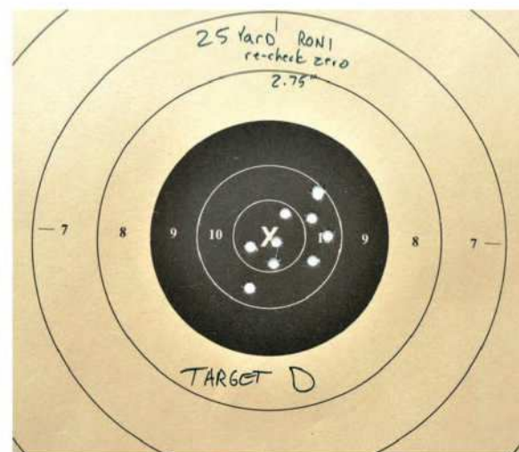
Target D: After removing and reinstalling the Glock 19 from the Micro RONI Stabilizer twice, Tarr checked the zero, and discovered it had shifted less than an inch at 25 yards.
