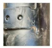
16 The new Monroe dampers go one better over the marks on the BMW (Sachs) originals. They have a welded on plate with a protruding tag that slots into the hub slot. Note that the Monroe part numbers end in L or R for left and right.
