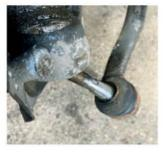
Remove the 18mm nut and split the steering arm to hub balljoint, either with a balljoint splitter or just clouting the hub arm with a steel hammer – don't go mad. The joint will pop out, retrieve the alloy washer if it falls out.
