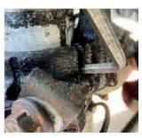
O Use an allen key in the hub slot, turn it to open up the slot and release tension on the strut. Spray plenty of penetrating oil into the gap (here, the strut has come out slightly). On RHD cars the line under 'R' must line up with the hub slot on the drivers wide, the 'l lines up with the slot on the passenger side.
