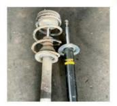
11 Here is the strut and the new Monroe replacement from GSF. The spring is quite rusty, I cleaned up the rust and painted them – E39 springs can snap and a rusty scab is as good a place as any for a break point.
