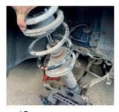
10 Support the hub on a block of wood or similar and withdraw the strut assembly from the hub. Use plenty of penetrating oil if needed and twist the strut around – they come out quite easily.
