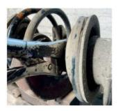
13 With the coil compressed enough, you can remove the 21mm top nut. You may find that the damper shaft spins so clamp it lightly at the top only. Do not clamp anywhere lower down on the shaft that may damage the damper seal if you are reusing the strut, i.e fitting lowering springs.
