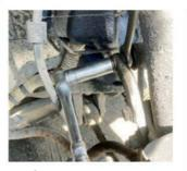
With the front wheels off and the car on axle stands, disconnect the anti-roll bar by holding the stud with a 16mm spanner and undoing the 16mm nut. With both wheels off there is no strain on the anti-roll bar and it's much easier.
