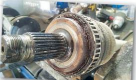
joint and it rusts, the resulting corrosion
