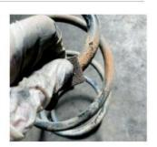
15 The spring was given a clean up on the rusty areas with both a wire brush in a bench grinder and also coarse wet and dry before being painted satin black. Ideally, tatty springs should be replaced and new ones from GSF are not dear - its Lesjofors spring range is extensive.
