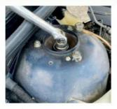
The first job is to slacken (but do not remove) this 21mm top nut. If you don't, it can be a bit difficult to remove later without an air gun. On reassembly it's torqued up to 44Nm on an M12 thread and 64Nm on an M14 thread.
