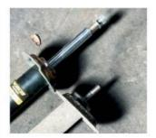
14 Yep, that one is dead. The chromed shaft was pushed in very easily with little resistance and did not rebound. It should be hard work to push the shaft down and it must always return fully.
