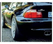
optimised the exhaust gas flow, improving the throttle response. In the handling department, stiffer Schnitzer springs were fitted with sports dampers from Bilstein, lowering the car by 25mm, which allowed for higher cornering speeds and more precise handling.
