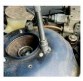
9 Up top remove the three 13mm strut top mounting nuts that are torqued to 24Nm. The strut will now drop down so move the steering arm out of the way and pull the strut out from the front arch.
