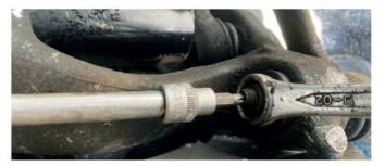
17 Reassembly is simple enough, but you must only torque the damper top nut and the suspension arm to subframe nut and bolt with the car on the ground or the suspension at normal ride height. I used a jack to raise the suspension. To re-tighten the steering arm nut (65Nm) you may have to hold the ball pin with a Torx of Allen socket as seen here.
