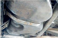
Below left: Compact's fuel tank retaining strap was replaced. Left: BBS alloys have been freshly powder coated too.
