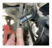
4 Now remove the two bolts seen here. The upper one is a 16mm that goes into the hub, the lower is a 16mm pinch bolt and 18 mm nut that clamps the strut into the hub. Note that the bolt can seize.
