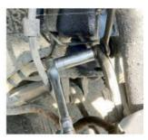
3 Remove the brake calliper from the carrier by unscrewing and removing the two sleeve bolts with a 5mm Allen socket as seen here. Remove the steel clip on the front of the calliper, push the pads away from the disc with a screwdriver and hang the calliper up on a bit of wire out of the way.
