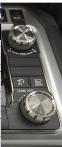
TWIST KNOBS Toyota's off-road gizmos such as Turn Assist are on the right side of the center console.
